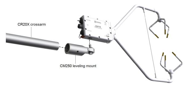
Figure 6-3. CSAT3B mounting
